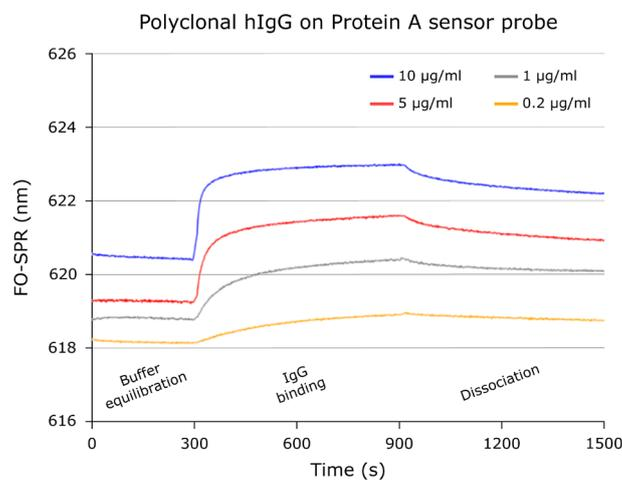
Figure 3. A sensorgram illustrating the responses generated by 4 different concentrations of hIgG ( $\mu\text{g/ml}$ ) on a Protein A sensor surface including buffer equilibration (baseline) and optional extended association and dissociation steps.
