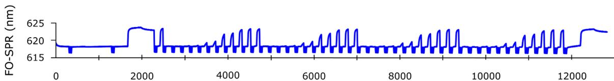
Figure 5: Results from a concentration screening including 48 regeneration cycles. The CV measured was less than 10%, generally presenting at around 2-5%. Screening cycles including regeneration used here were performed in less than 4 minutes per sample. Actual binding measurement for concentration determination took 60 seconds per sample.
