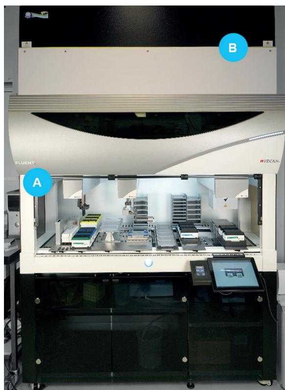
Figure 1: A Fluor Automation Workstation (A) fitted with a vertical laminar flow HEPA hood (B) used for the cell seeding and medium exchanges.
