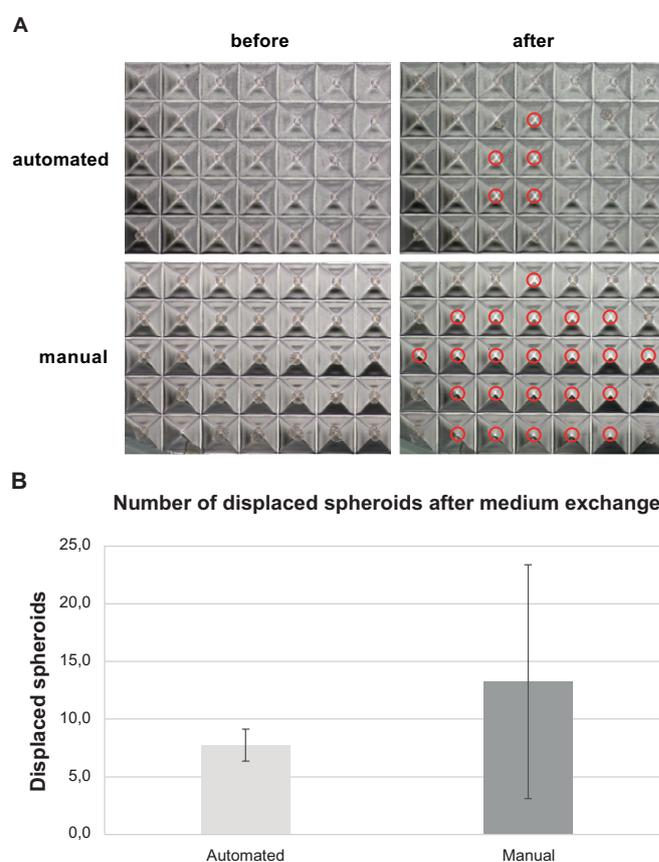
Figure 3: Image analysis before (A, left) and after (A, right) medium exchange revealed fewer displaced spheroids (○ red circles) per well using automation. Smaller error bars also indicate better reproducibility and consistency for the automated protocol (B).
